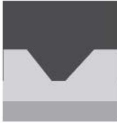
This method for 90° folds may lead to dimensional variations of  $\pm 1.0\text{mm}$  and these should be compensated for in the panel size calculations.
